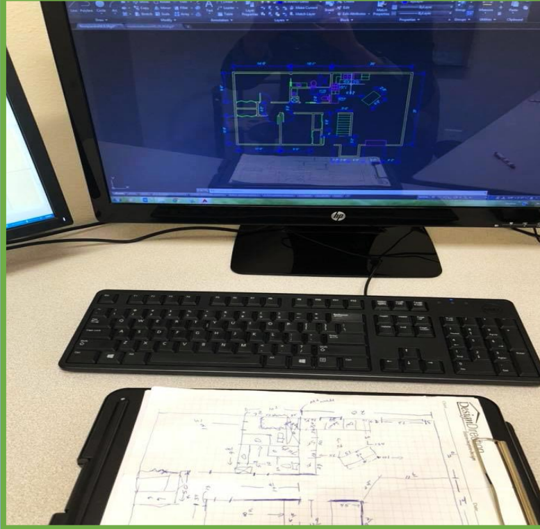
Transferring sketched floorplan from site measurement to AutoCad.
